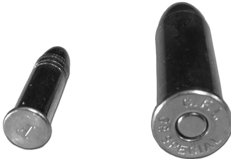
Rimfire vs. centerfire cartridges. At left is a .22 Long Rifle round, a rimfire cartridge. At right is a .38 Smith & Wesson round, a centerfire cartridge, seen from below. Note the telltale, circular primer cup that sits at the bottom of the centerfire cartridge's case head. The rimfire cartridge lacks this. Instead, it has a layer of priming compound (not visible) applied to the inside of the brass rim of the cartridge.
