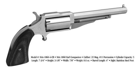
This North American Arms revolver is a muzzleloader. To load the gun, one removes the revolving cylinder from the frame of the gun. After that, one rams gunpowder and then a bullet into each of the five cylinder chambers, from the front. Finally, one places percussion caps on the back of each cylinder chamber, and then puts the cylinder back into the gun.
