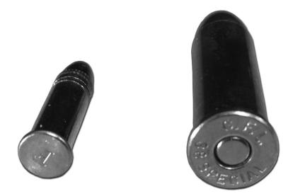
Rimfire vs. centerfire cartridges. At left is a round of .22 Long Rifle, a rimfire cartridge. At right is a round of .38 Special, a centerfire cartridge, seen from below. Note the telltale, circular primer cup that sits at the bottom of the centerfire cartridge's case head. The rimfire cartridge lacks this. Instead, it has a layer of priming compound (not visible) applied to the inside of the brass rim of the cartridge.
