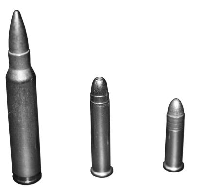
Different types of ammunition. From left to right, .223 Remington, .22 WMR, and .22 LR. Note that the bullet (the top part) for the .223 Remington is only 3/1000 of an inch wider than the .22 caliber bullets. But the .223 Remington's case is much wider and larger, allowing more room for gun powder, making it far more powerful than the other two.
