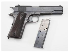
Colt 1911 semi-automatic pistol, with seven-round magazine. This specimen was manufactured in 1918, and used by the U.S. Army in World War I and World War II. The openings in the magazine side are "witness holes," so that the user can see how many rounds are in the magazine when loading it.
