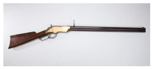
The 1860 Henry lever action rifle. This specimen was manufactured 1864. The lever is the oval that attaches to the trigger guard. The oval and the guard move as a unit, swung down to eject, then up to reload. The pivot is at the top front of the trigger guard. The rifle is still in production today, with modifications for modern ammunition.
